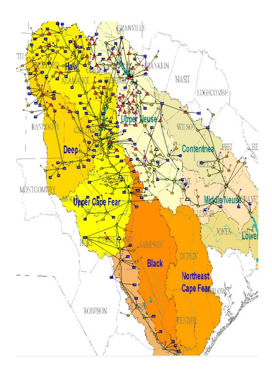
The user can click on any node or connecting arc on the schematic to access specific information, like reservoir elevation-storage-area data or minimum streamflow requirements. These data are also contained in tables contained on other tabs of the model.
