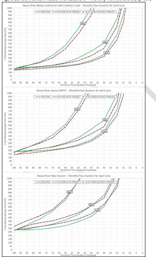
Figure 22. Downstream Neuse River Locations -- Monthly Flow Durations (Apr-Jun)
