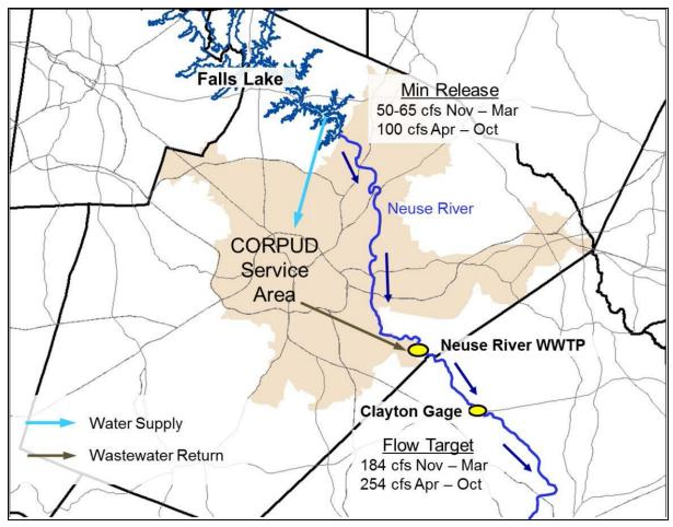
Figure 3.1 - Schematic of Features between Falls Lake and Clayton, NC
