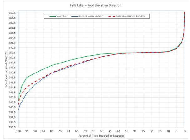
Figure 8. Falls Lake Pool Elevation Duration for All Model Conditions
