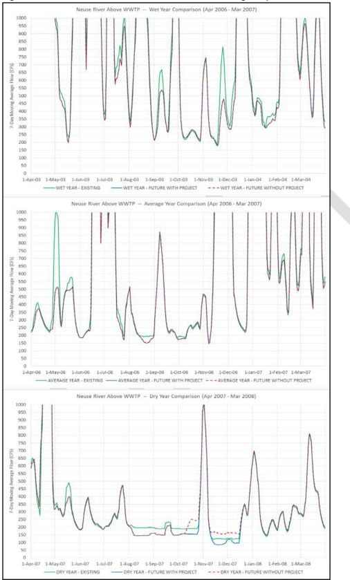
Figure 19. Neuse River Flow Above WWTP for Wet, Average, Dry Years
